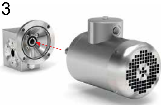
Fit the motor on the gearbox paying attention to the correct position of the O-ring.
