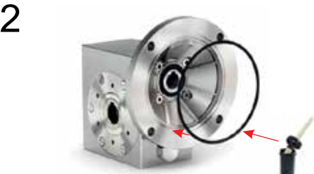
An o-ring must be installed in the input flange of the gearbox to ensure a water tight seal between the motor and the gearbox. This O-ring is provided in a bag which is attached to each and every gearbox. To hold the O-ring in place use Loctite SI 5699 sealant grey paste or food grade grease.
